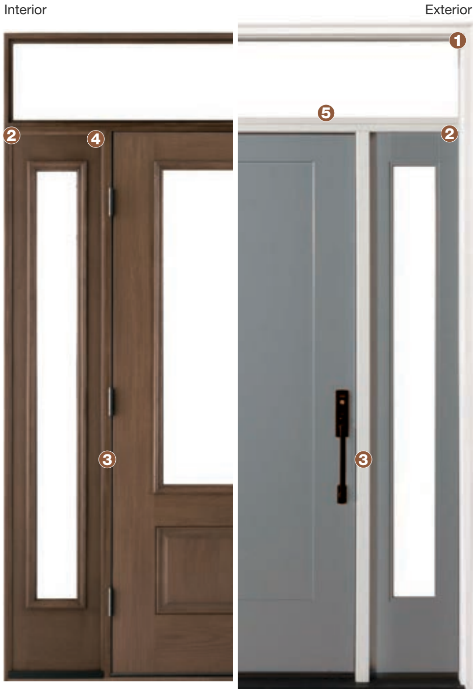
1 Brickmould 2 Jamb 3 Mullions 4 Cove Mould 5 Transom Sill
